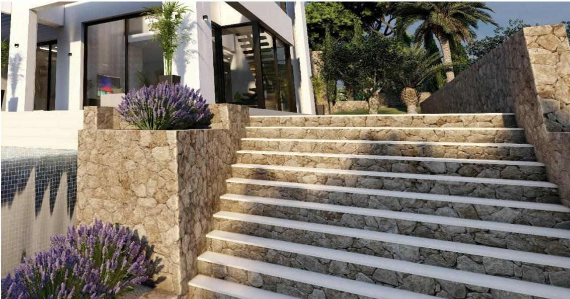
*Interior steps on the plot formed by white concrete plates separated by a white micro-gravel joint. Garden walls in dry stone masonry, formation of garden stairs with tread made of limestone or white concrete and masonry partition.*
